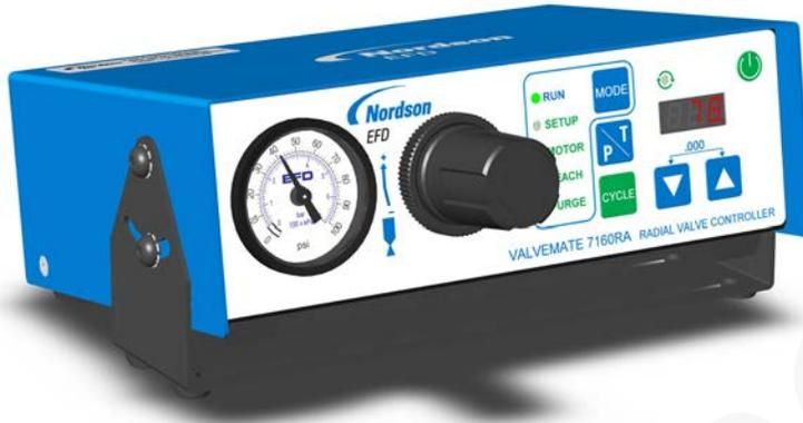
Use the universal mounting bracket (included) to mount the controller either over or under the cabinet. The bracket allows the controller to pivot 30 degrees from a horizontal position. When mounted under a workbench, secure with screws or nuts and bolts to support 6 kg (14 lb).
