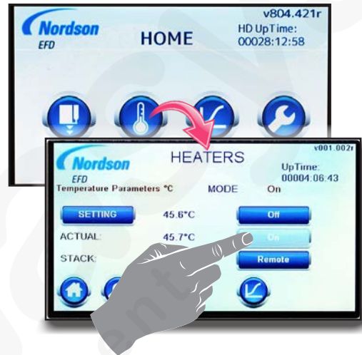
Switching on heater control
