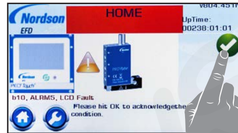
Clearing an alarm
