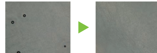
Under atmospheric pressure, 2 min mixing and degassing
