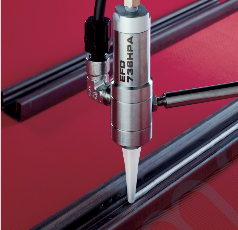
Apply RTV to automotive valve covers.
