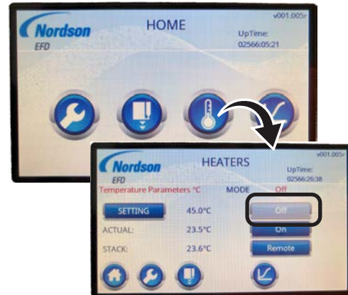
Switching OFF heater control
