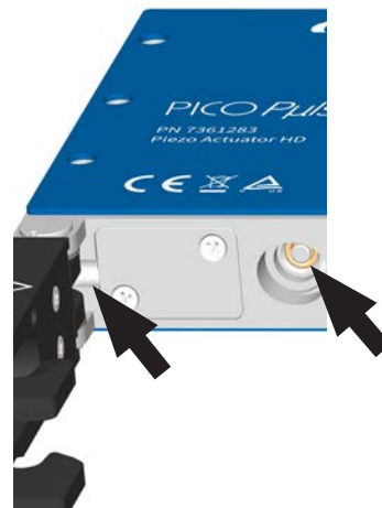
Piezo actuator cleaning locations (do not use sharp tools)
