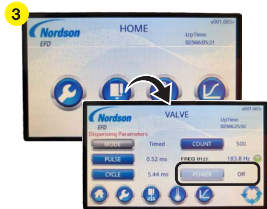
Switching valve POWER to OFF (standard Touch controller VALVE screen shown)
