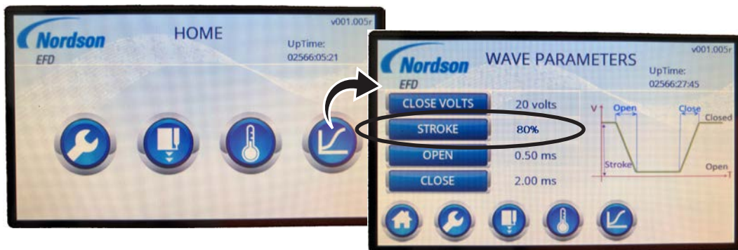
Wave Parameters screen on the standard Touch controller (STROKE units set in percentage of CLOSE VOLTS)
