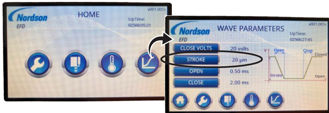
WAVE PARAMETERS screen on the Touch XP controller (STROKE units set in microns)
