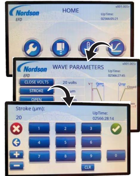
Adjusting the STROKE setting of the enabled wave profile (Touch XP controller)
